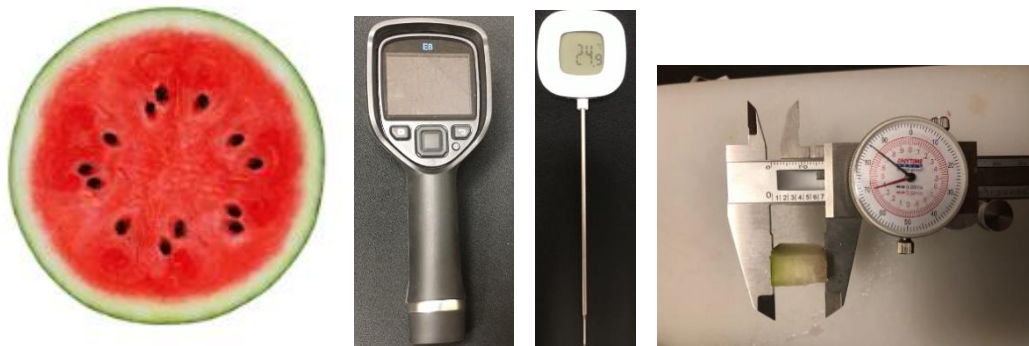
Fig. 1 The experimental setup used to take the temperature measurement across the radius of the fruit.
