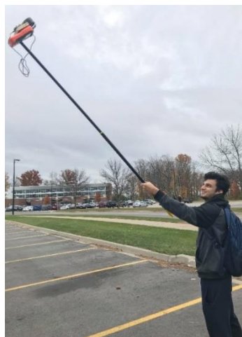
Fig. 1 Thermo-anemometer holding frame for far-reaching positioned vents
